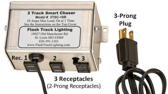
Keep in mind that a typical household circuit and receptacle is only rated at 15 amps. (This should not be a problem, since this controller is only rated for up to 10 amps.)
